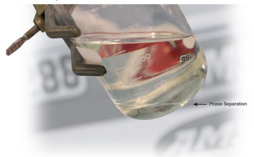
When ethanol/water mixtures fall to the bottom of fuel containers, it leads to lean-burn situations. Quickshot helps keep water molecules dispersed to prevent phase separation.
